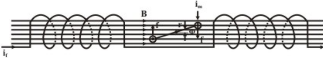
Fig. 43.1(b): Magnetic - field and torque developed in moving coil of an electro dynameter.
