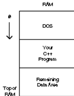
Figure 1.6. After MS-DOS and a C++ program, there is less RAM for data.
